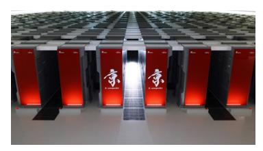
K computer: 8 core CPU x 82944 node system with peak performance of 10.6 PFLOPS
