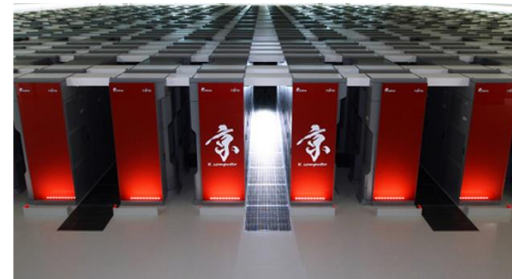
K computer: 8 core CPU x 82944 node system with peak performance of 10.6 PFLOPS
